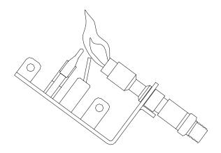
FIGURE 10. Incorrect Shape of Pilot Flame
